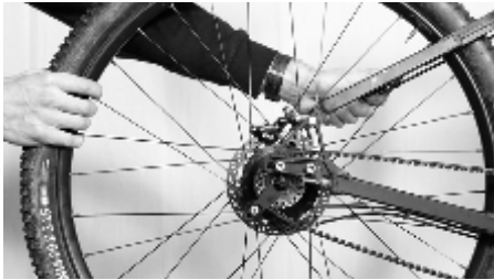
Illustration 3: Correct alignment of the belt
