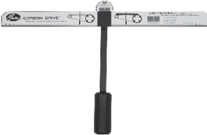
Illustration 3: Eco Tension Tester in use
