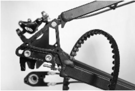
Illustration 1: Opening the frame to mount the belt
