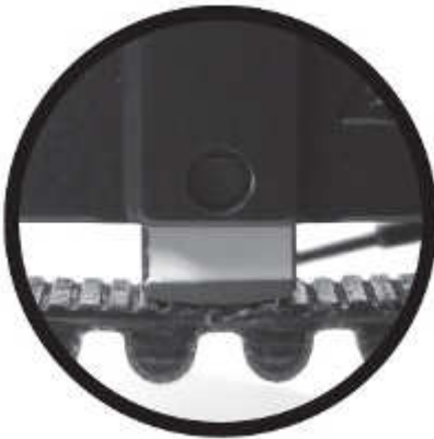
Illustration 3: Optimal belt tension
