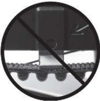
Illustration 1: Incorrect belt tension
