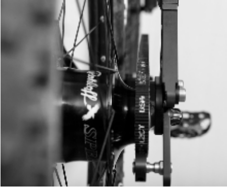
Illustration 3: Correct alignment of the belt
