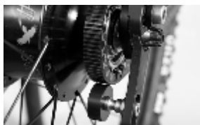
Illustration 1: Rohloff SPEEDHUB 500/14 with Snubber
